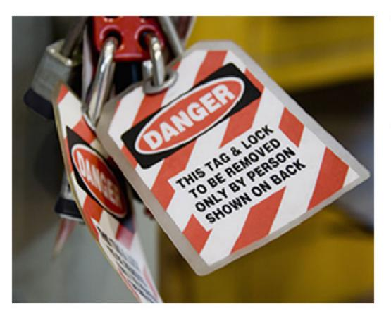
To accomplish this objective, the standard requirements include the establishment of an energy control program that consists of specific energy control procedures, employee training, and periodic inspections to ensure that before service and maintenance is performed, machines and equipment that could unexpectedly startup, become energized, or release stored energy, are isolated from their energy source(s) and rendered safe for further work on them.
