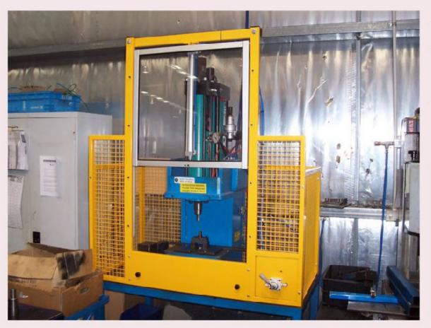
Another potential application of this type of guard is where the gate is a component of a perimeter safeguarding system. Here, the gate may provide protection not only to the operator but pedestrian traffic as well.
