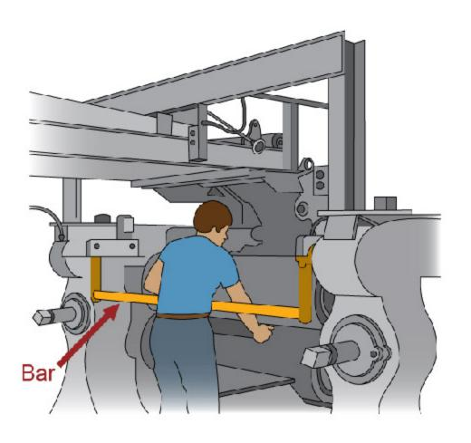
The safeguards for electromechanical devices include the contact bar or probe that travels a predetermined distance between the operator and the danger area, with interruption of this movement preventing the starting of the machine cycle. Advantages and limitations include:
