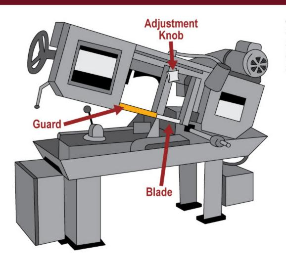
Adjustable guards are useful because they allow flexibility in accommodating various sizes of stock. This type of guard provides a barrier that may be adjusted to facilitate a variety of production operations. With this, adjustable guards have the following advantages and limitations:
