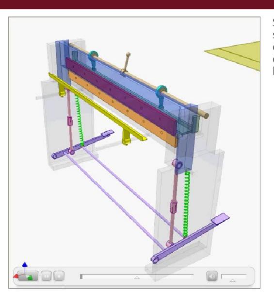
Shearing action involves applying power to a slide or knife to trim or shear metal or other materials. A hazard occurs at the point of operation where the stock is inserted, held, and withdrawn. Examples of machines used for shearing operations are mechanically, hydraulically, or pneumatically-powered shears.
