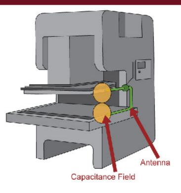
The radiofrequency (capacitance) presence-sending device uses a radio beam that is part of the machine control circuit. When the capacitance field is broken, the machine will stop or will not activate. Like the photoelectric device, this device should only be used on machines which can be stopped before the employee can reach the danger area. This requires the machine to have a friction clutch or other reliable means for stopping.
