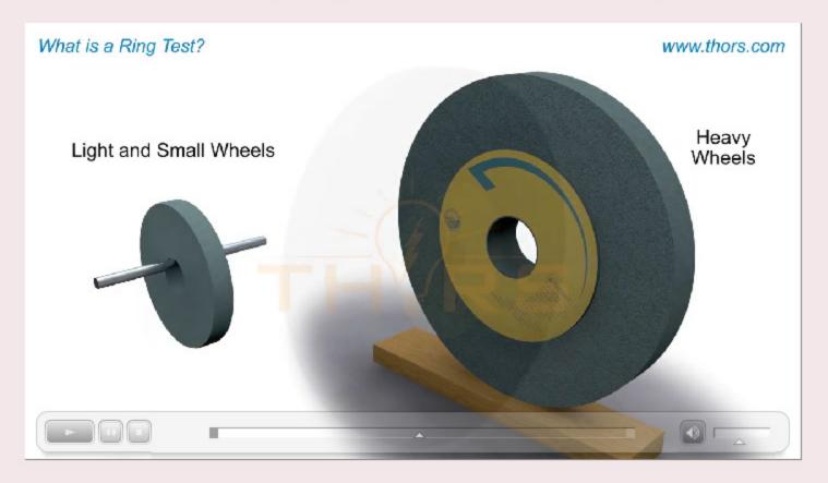
when applying the ring test. Otherwise the sound will be deadened. It should also be noted that organic bonded wheels do not emit the same clear metallic ring as do other types of wheels. Click play to see how a ring test is conducted.
