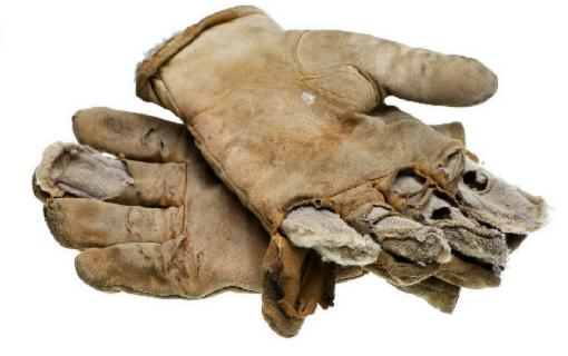
With these types of degradation, penetration may be allowed, and permeation could be enhanced or restricted which may ultimately compromise the protective nature of the glove, placing the employee at risk for a potentially serious hazard.
