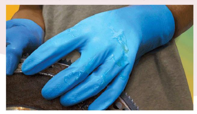
the greater the breakthrough time, the more protective the material is for that particular substance. However, it is to be noted that factors such as temperature, pressure and perspiration within the glove may enhance permeation, thereby reducing the breakthrough time and the protective measures of the glove. The maximum breakthrough time is 480 minutes, equivalent to an 8-hour day.
